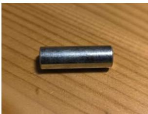
I attach these to a soft iron **magnetic coil core** (thickness=8 mm / length=25 mm) ([example](#)), which costs around 2 Euros for a pack of 10.
