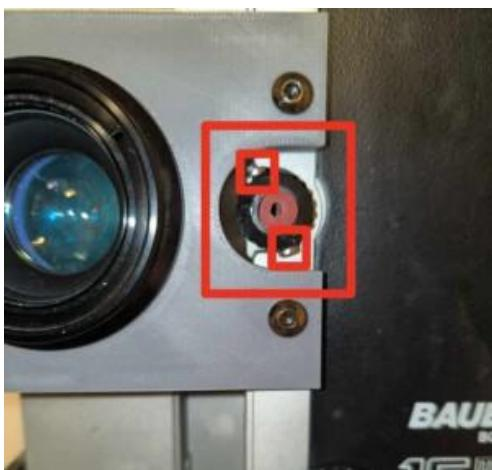
Because it has already proven itself with the Syncino and I don't want any internal installations, the neodymium magnets were attached to the handwheel of my Bauer P8 TS using mounting adhesive or superglue.
